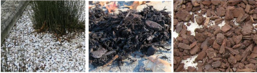
Non-floating mulches include shell (left, Nelson port) and composted, stringy bark (centre, Stoke). Bark nuggets (right) should never be used where water will float or pond as they are prone to floating.
