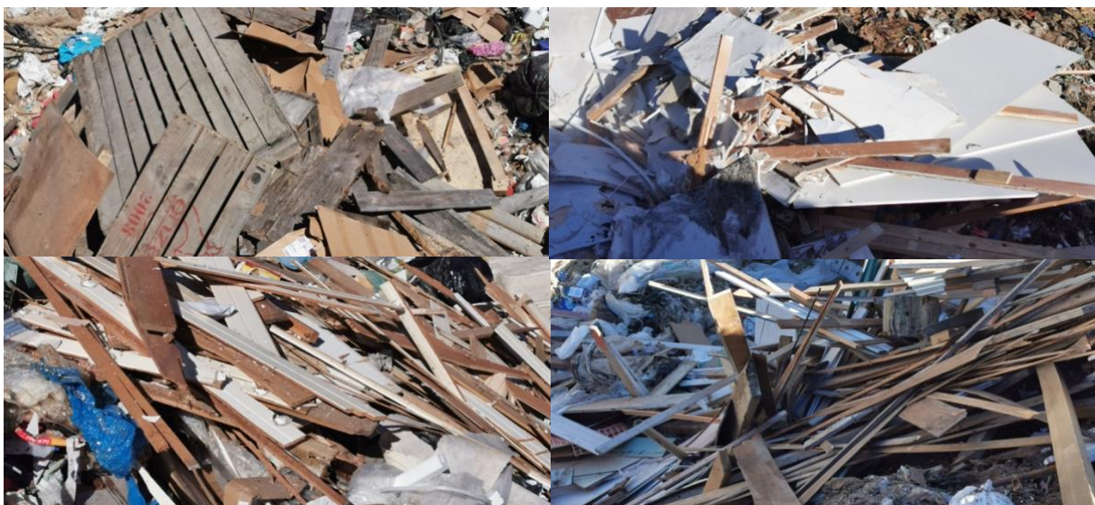
Figure 4. Examples of timber waste.
