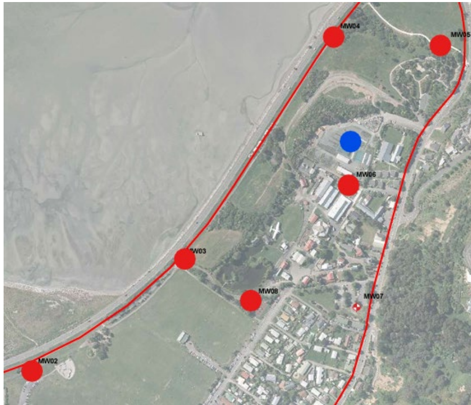
Figure 21: Wells (red) which consistently demonstrate elevated levels and (blue) site of weekly testing for airborne gas.
