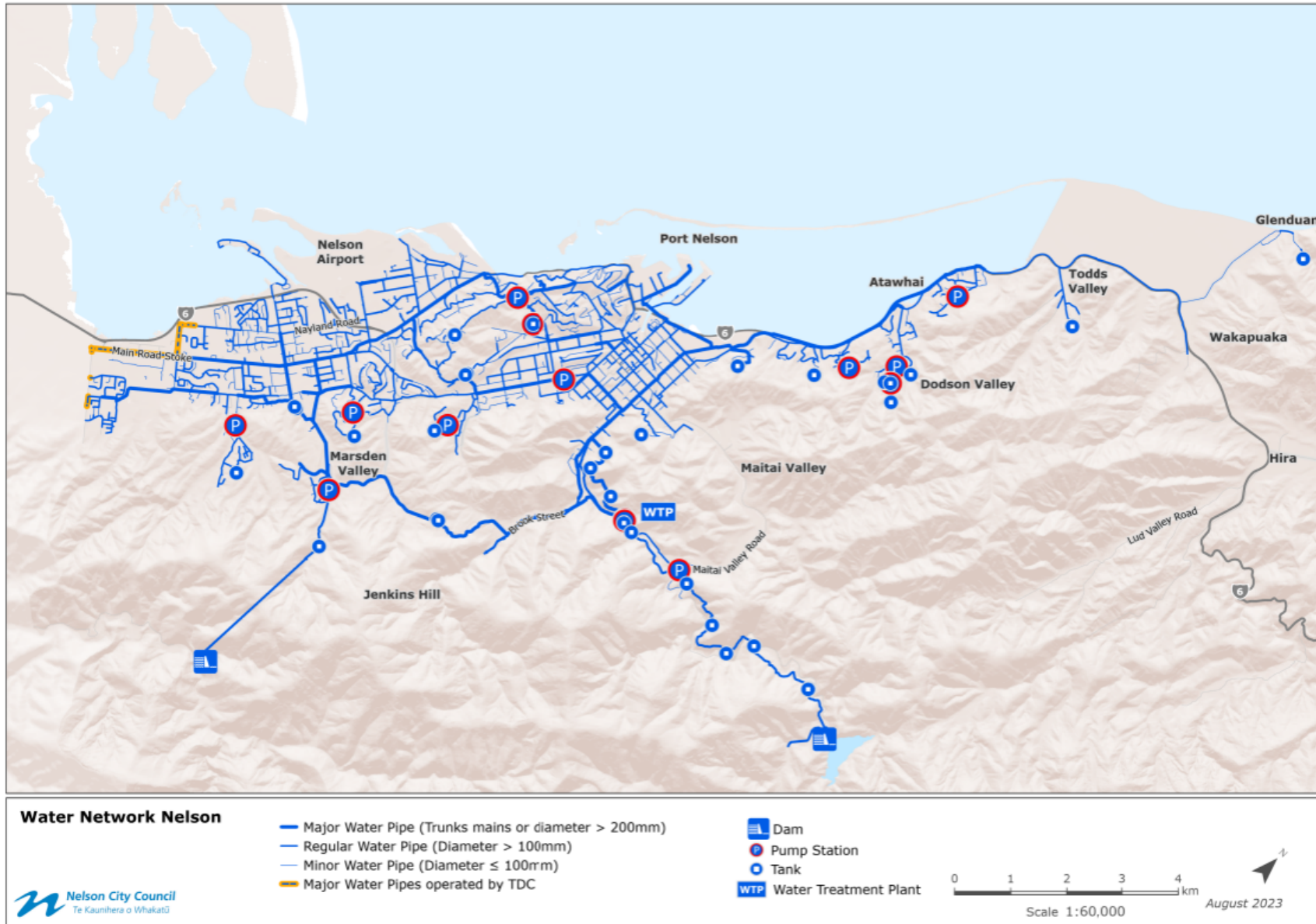
Figure 1-1: Water Network Nelson
